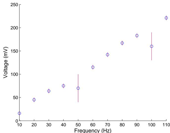
Figure 1: The signal to noise ratio from a frequency to voltage converter diminishes near harmonics of the main frequency.
