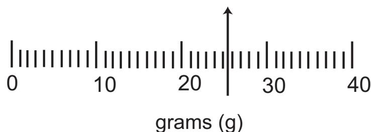
FIG. 2: An analog reading displayed on an analog balance.
