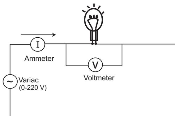
FIG. 2: A schematic diagram of the experiment.
