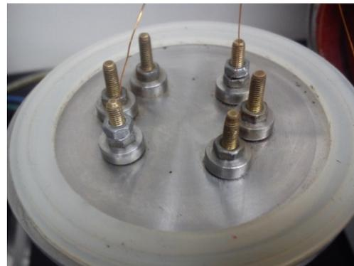
Insert the sample along with the high temperature sleeve in the tube, the position of the sample is shown in the figure below. (The sample should be placed close to the thermocouple of the furnace). Close the end with the feed through by clamp. Close the furnace.
