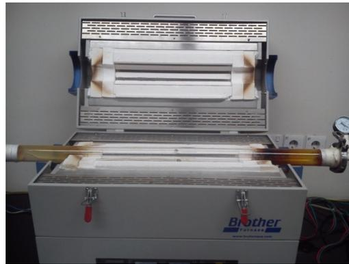
Remove the clamp on the feed through, by holding the feed through, and remove it from the tube end.
