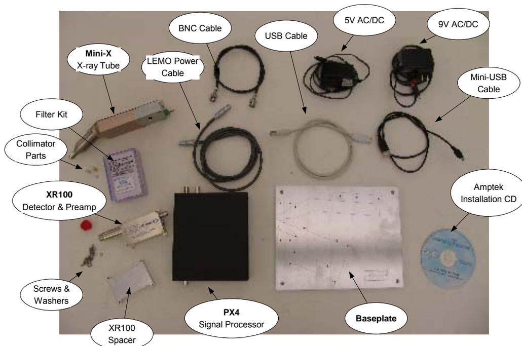
Figure 1-1. Photograph of Amptek components
