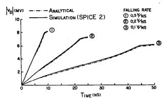
Fig. 3. Comparison of the analytic and computer simulated transient responses for three different gate voltage falling rates. The parameters for Figs. 3 and 4 are  $V_S = 0$ ,  $C_L = 2$  pF,  $V_{T0} = 0.60$  v,  $W = 4 \ \mu m$ ,  $L = 3.3 \ \mu m$ ,  $L_D = 0.35 \ \mu m$ , and  $\beta = 30.3 \ \mu A \cdot V^{-2}$ .
