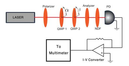
Figure 1: The polarizer and analyzer are oriented along the same direction. The retarders QWP 1 and QWP 2 are at  $\alpha$  and  $\beta$  with respect to the first polarizer respectively. The red line shows the perceived path of laser.
