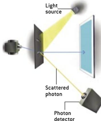
The fringes do not appear if the particles interact with something that could thereby be used to ascertain each particle's location at the slits. For example, a photon of light (*yellow line*) might scatter from the particle and reveal that it went through the right-hand slit. The photon need not be detected—all that matters is that the "which slit?" information in principle could be determined if it were to be detected.
