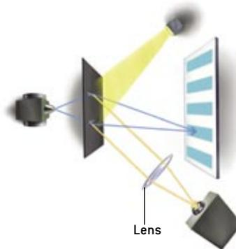
A quantum eraser erases the "which slit?" information. If the particle scatters a photon, a lens could make it impossible to ascertain which slit the photon came from. In that case, the corresponding particle apparently goes through both slits, as before, and fringes can be observed. The strangest feature of this quantum erasing is that the behavior of the particle at the slits seemingly depends on what the photon encounters *after* the particle has passed through the slit(s).
