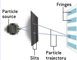
Particles sent through two slits generate bands (called fringes) on a detector screen when large numbers arrive at some regions (*blue*) and very few arrive at other regions (*white*). This interference pattern arises only if each particle could have traveled through both slits to arrive at the screen (*arrows*).
