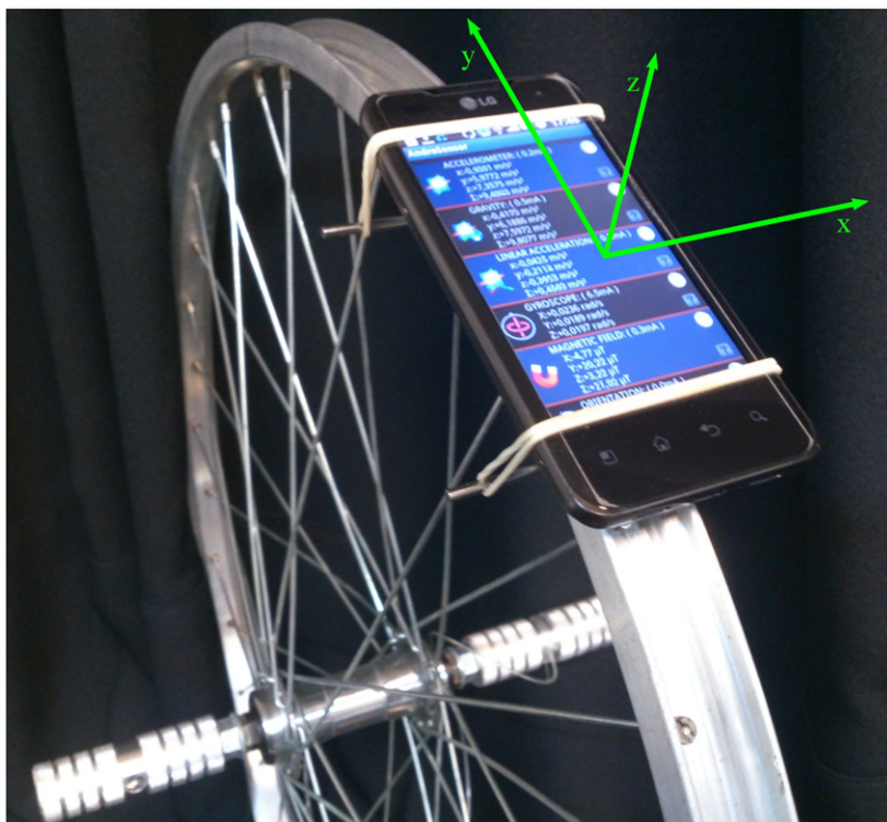
Figure 1. Smartphone mounted on a bike wheel moving in a vertical plane and a scheme indicating the axes orientation.
