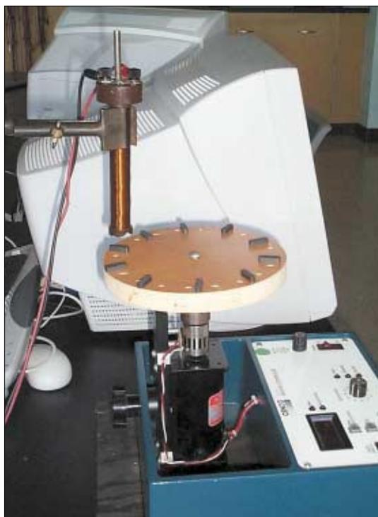
**Fig. 1. Scaled-up model of the hard drive's platter (disk) and inductive "read" head (solenoid). Permanent magnets at edge of platter store the information. When the disk is spun, an emf is induced in the solenoid and recorded by the computer.**
