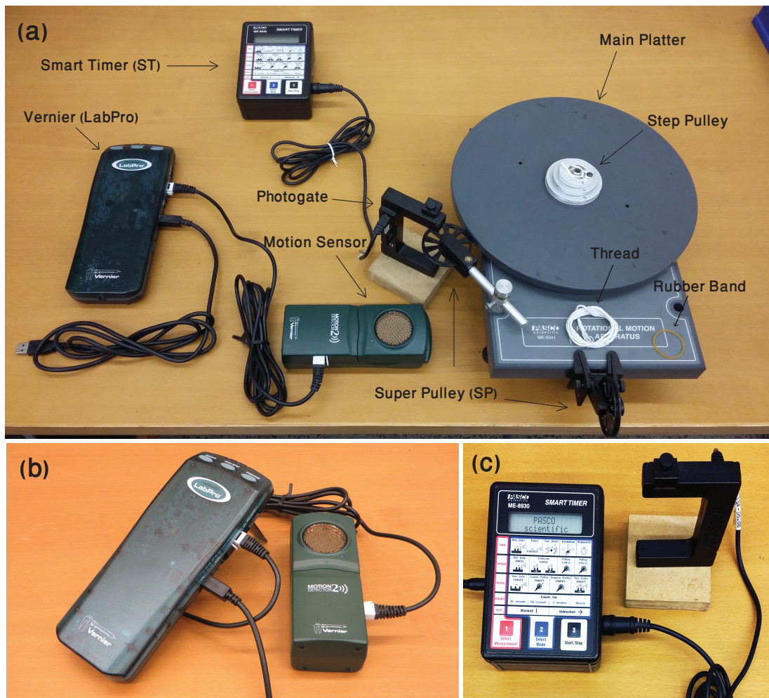
Figure 3: (a) The components of the rotational motion apparatus. Note the arrows showing the particulars of the components, (b) Vernier's LabPro and Ultrasonic Motion Detector (MD-BTD), (c) PASCO's (ME-8930) Smart Timer.
