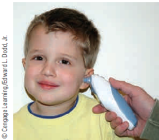
Figure 40.8 An ear thermometer measures a patient's temperature by detecting the intensity of infrared radiation leaving the eardrum.
