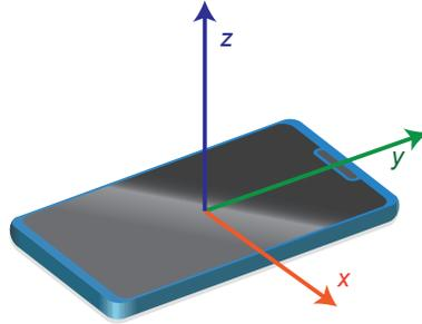
Figure 2: The conventional orientation of the smartphone's axes, used by its internal sensors. For example,  $\omega_z$  will represent angular speed of the phone as it rotates about an axis perpendicular to its own plane (the  $z$  axis), and  $a_x$  will be its acceleration parallel to the smaller width, *etc.*
