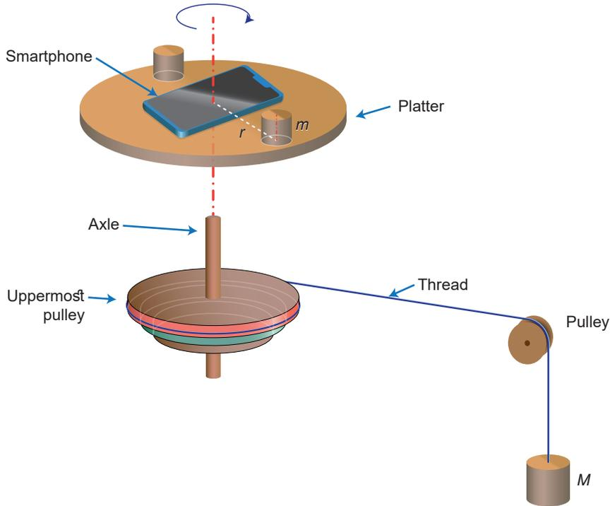
Figure 3: Scheme of the experiment is depicted here. Various parts have been labelled.
