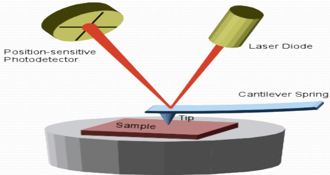
Surface information is revealed by raster scanning a cantilever probe in close proximity with the sample surface and probe sample interaction is monitored.
