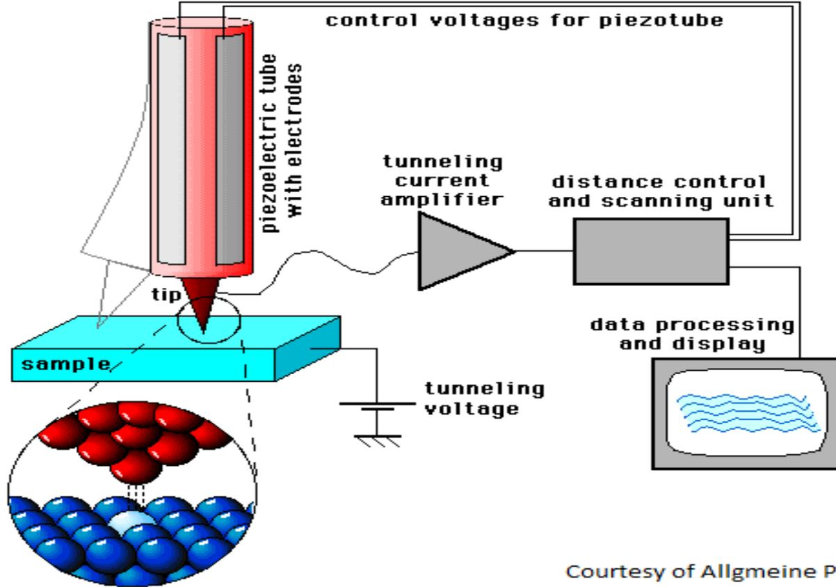
A potential difference is applied on the sample surface and a conducting tip is brought very close to that surface which allows electric current to tunnel through the gap.
