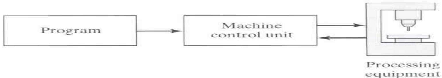
Figure 6.1 Basic components of an NC system.
