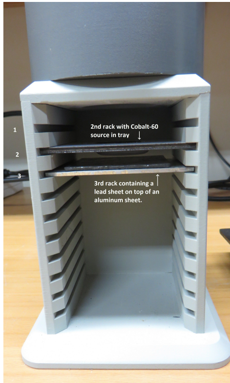
Figure 8: The source is kept on its tray on the second rack in the shelf. The lead sheet for enhanced backscattering is kept on an aluminum sheet which is kept on the third rack in the shelf.
