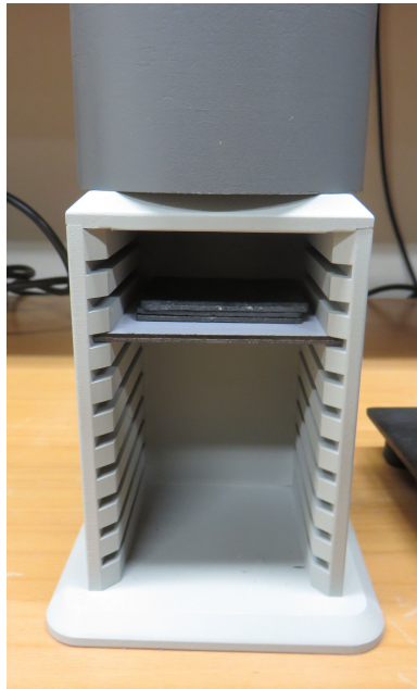
Figure 14: The source has been kept on its tray in the third rack. Three lead plates placed on the source for attenuation of gamma rays are also visible.
