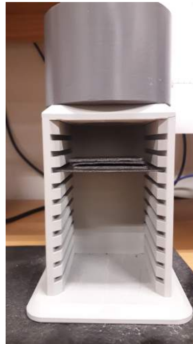
Figure 4: Lead sheets serve as photon absorbers in the mass attenuation coefficient test
