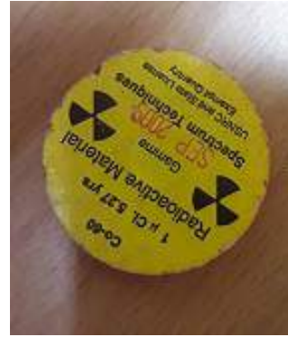
Figure 2: Co-60 source with half-life of 5.27 years and decay rate of 1 Ci ( 1\text{Ci} = 3.7 \times 10^4 counts/s)
