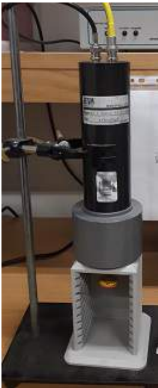
Figure 3: REXON NAI 1.50PX1.50/2.0LV detector with cylindrical lead shielding and photo-multiplier tube. The detector is perched on a stand closed on three sides. The slots in the stand are used to vary the distance of the source from the detector. Source is placed in a tray on one of the level.
