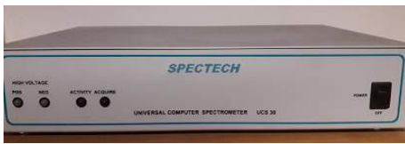
Figure 1: Spectech Multi-channel analyzer
