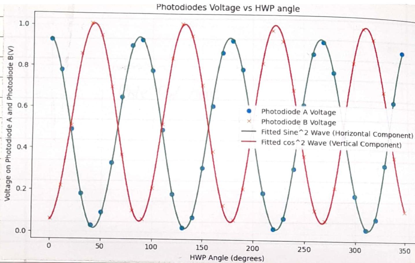
The figure illustrates the experimental data as well as the fitted  $\sin^2$  and  $\cos^2$  functions for the horizontal and vertical components of the light.
