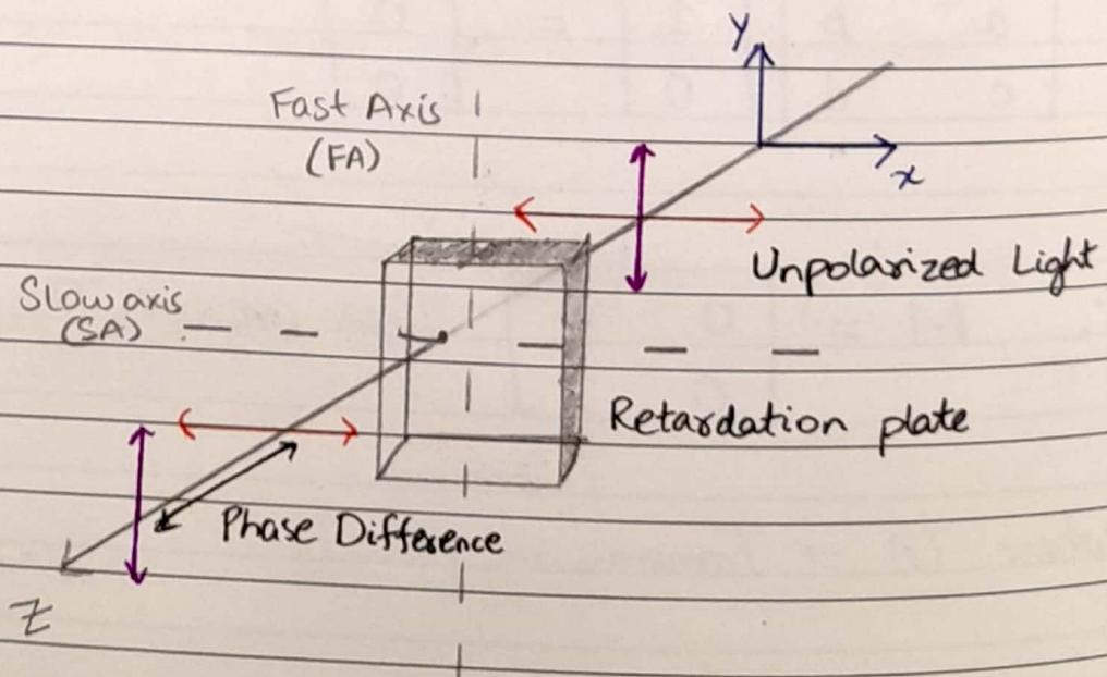
When the net phase difference  $\Delta\phi = \frac{\pi}{2}$ , the retardation plate is called a quarter wave plate.
