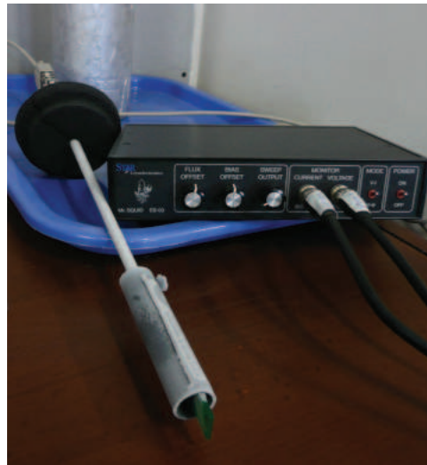
Figure 11: Photograph of the Mr. SQUID probe along with its electronic box.
