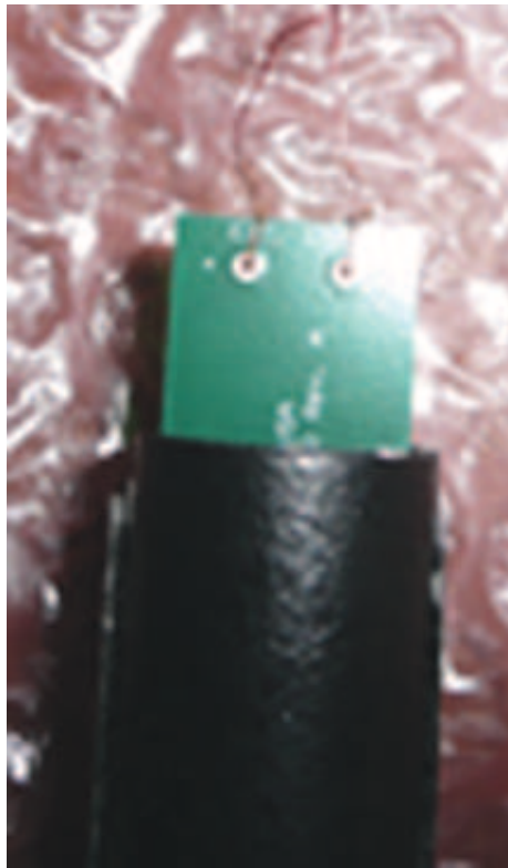
Figure 25: Copper wire connection to the EXT. COIL terminals to find its the coil's resistance at liquid nitrogen temperature.
