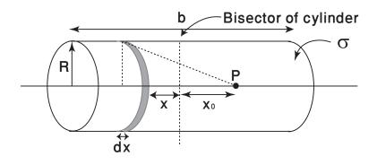
Consider a point P at a distance  $x_0$  from the transverse bisector of the cylinder. Consider a thin strip at a distance x from the bisector. This strip results in a potential,
