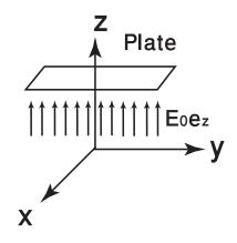
Suppose the plate is horizontal (parallel to xy) and the electric field is vertically upward. We have  $\mathbf{E} = E_0 \hat{\mathbf{e}}_z$ . We can compute the elements of the stress tensor.
