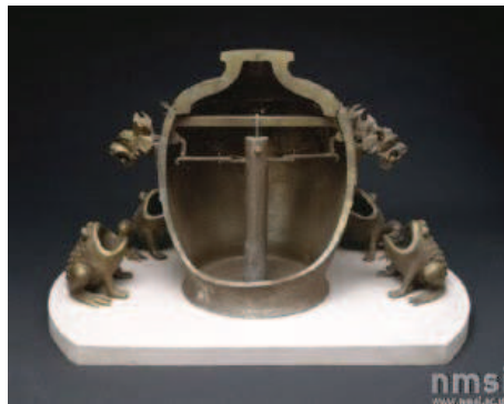
Figure 1: Zhang Heng's seismoscope, the first device to detect an earthquake [3].
