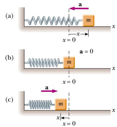
**Figure 13.5** A block of mass  $m$  attached to a spring on a frictionless surface undergoes simple harmonic motion. (a) When the block is displaced to the right of equilibrium, the displacement is positive and the acceleration is negative. (b) At the equilibrium position,  $x = 0$ , the acceleration is zero and the speed is a maximum. (c) When the block is displaced to the left of equilibrium, the displacement is negative and the acceleration is positive.
