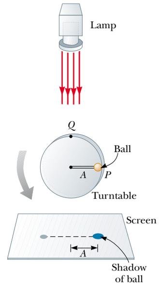
**Figure 13.17** An experimental setup for demonstrating the connection between simple harmonic motion and uniform circular motion. As the ball rotates on the turntable with constant angular speed, its shadow on the screen moves back and forth in simple harmonic motion.
