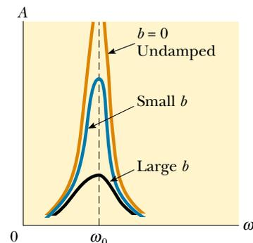
**Figure 13.22** Graph of amplitude versus frequency for a damped oscillator when a periodic driving force is present. When the frequency of the driving force equals the natural frequency  $\omega_0$ , resonance occurs. Note that the shape of the resonance curve depends on the size of the damping coefficient  $b$ .
