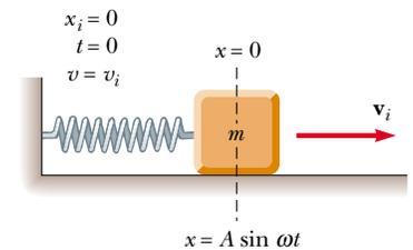
**Figure 13.8** The block–spring system starts its motion at the equilibrium position at  $t = 0$ . If its initial velocity is  $v_i$  to the right, the block's  $x$  coordinate varies as  $x = (v_i/\omega) \sin \omega t$ .
