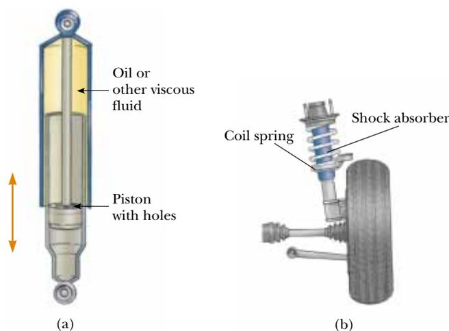
**Figure 13.21** (a) A shock absorber consists of a piston oscillating in a chamber filled with oil. As the piston oscillates, the oil is squeezed through holes between the piston and the chamber, causing a damping of the piston's oscillations. (b) One type of automotive suspension system, in which a shock absorber is placed inside a coil spring at each wheel.
