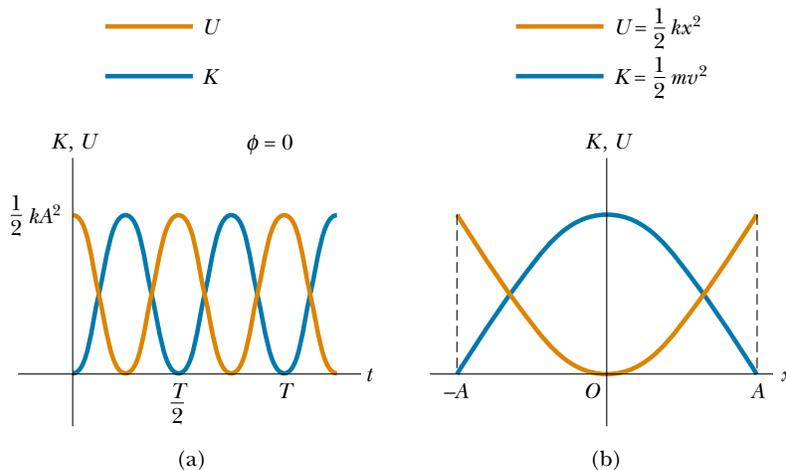
**Figure 13.9** (a) Kinetic energy and potential energy versus time for a simple harmonic oscillator with  $\phi = 0$ . (b) Kinetic energy and potential energy versus displacement for a simple harmonic oscillator. In either plot, note that  $K + U = \text{constant}$ .
