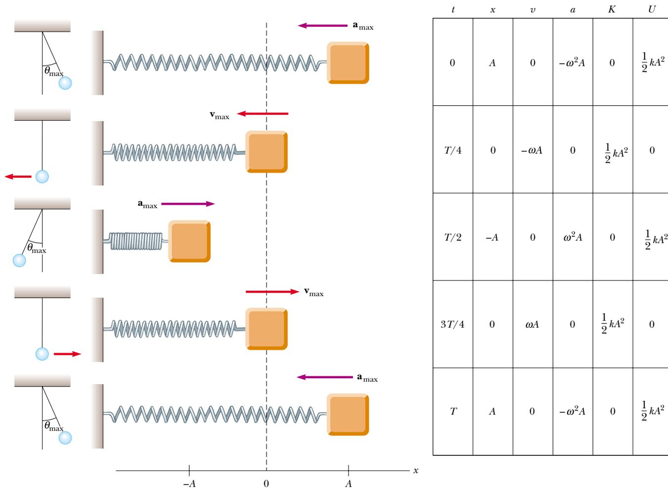
**Figure 13.10** Simple harmonic motion for a block–spring system and its relationship to the motion of a simple pendulum. The parameters in the table refer to the block–spring system, assuming that  $x = A$  at  $t = 0$ ; thus,  $x = A \cos \omega t$  (see Special Case 1).
