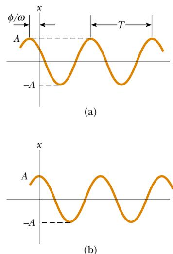
**Figure 13.3** (a) An  $x-t$  curve for a particle undergoing simple harmonic motion. The amplitude of the motion is  $A$ , the period is  $T$ , and the phase constant is  $\phi$ . (b) The  $x-t$  curve in the special case in which  $x = A$  at  $t = 0$  and hence  $\phi = 0$ .
