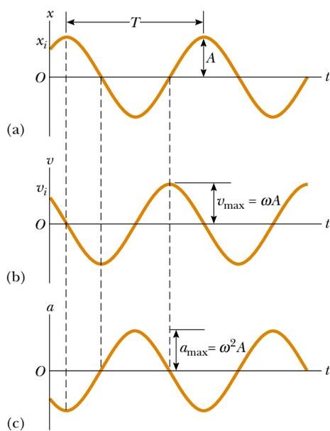
**Figure 13.4** Graphical representation of simple harmonic motion. (a) Displacement versus time. (b) Velocity versus time. (c) Acceleration versus time. Note that at any specified time the velocity is  $90^\circ$  out of phase with the displacement and the acceleration is  $180^\circ$  out of phase with the displacement.
