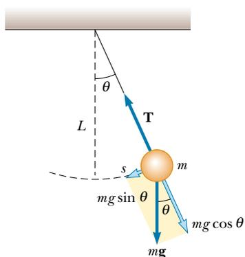
**Figure 13.12** When  $\theta$  is small, a simple pendulum oscillates in simple harmonic motion about the equilibrium position  $\theta = 0$ . The restoring force is  $mg \sin \theta$ , the component of the gravitational force tangent to the arc.
