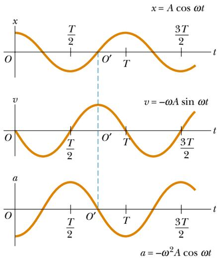
**Figure 13.7** Displacement, velocity, and acceleration versus time for a block–spring system like the one shown in Figure 13.6, undergoing simple harmonic motion under the initial conditions that at  $t = 0$ ,  $x_i = A$  and  $v_i = 0$  (Special Case 1). The origins at  $O'$  correspond to Special Case 2, the block–spring system under the initial conditions shown in Figure 13.8.
