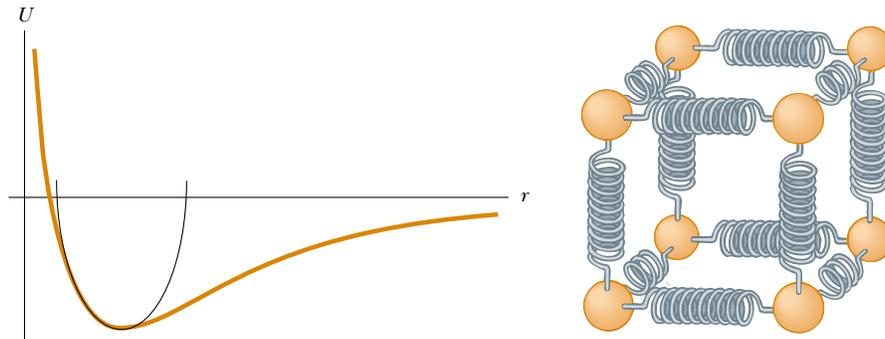
**Figure 13.11** (a) If the atoms in a molecule do not move too far from their equilibrium positions, a graph of potential energy versus separation distance between atoms is similar to the graph of potential energy versus position for a simple harmonic oscillator. (b) Tiny springs approximate the forces holding atoms together.
