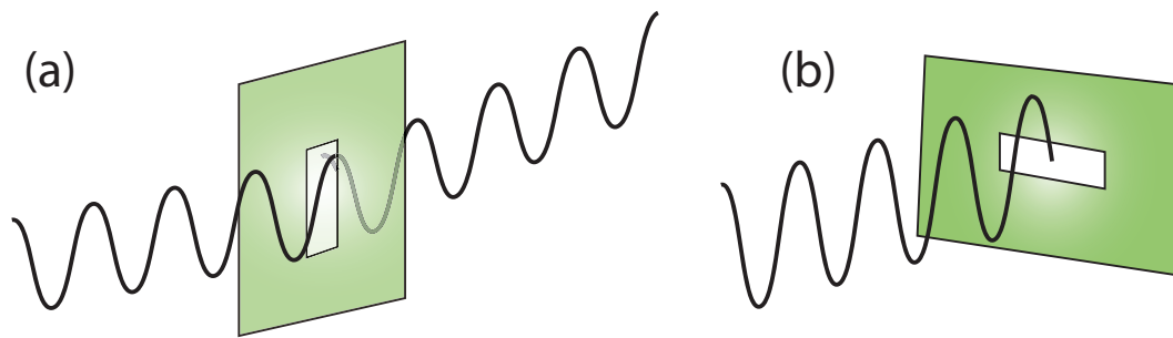
Figure 3: In diagram (a) a transverse wave is propagating towards a slit which is parallel to the motion of the wave hence allowing the wave to pass through whereas in (b) the wave gets blocked as its direction of motion is perpendicular to the slit axis.
