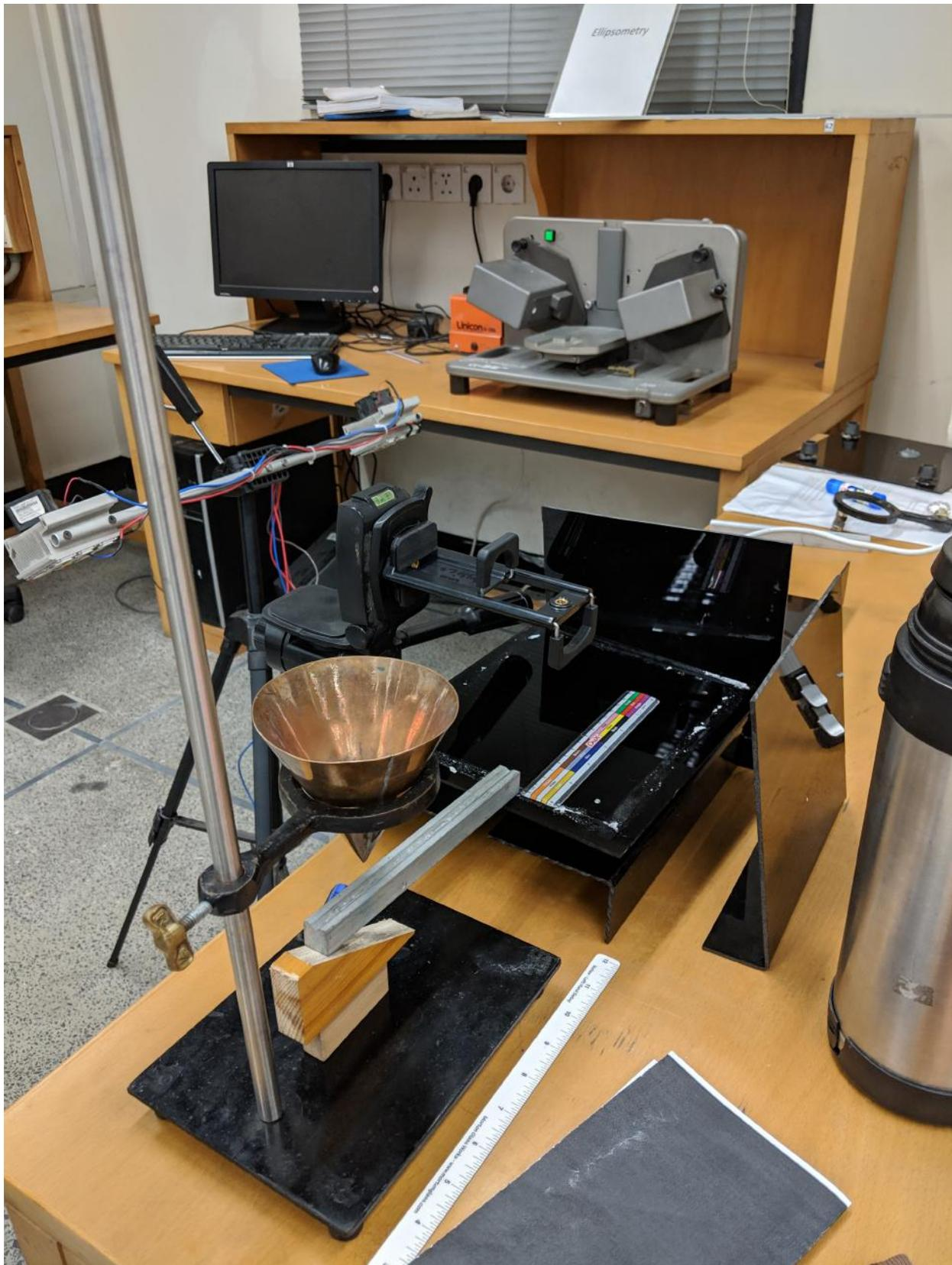
**Fig. 4.** The optimal setup looks like this. The light points downward to avoid reflections and glares. The plastic sheets are placed to reflect light from a range of angles. The ruler provides reference for calibration during tracking.
