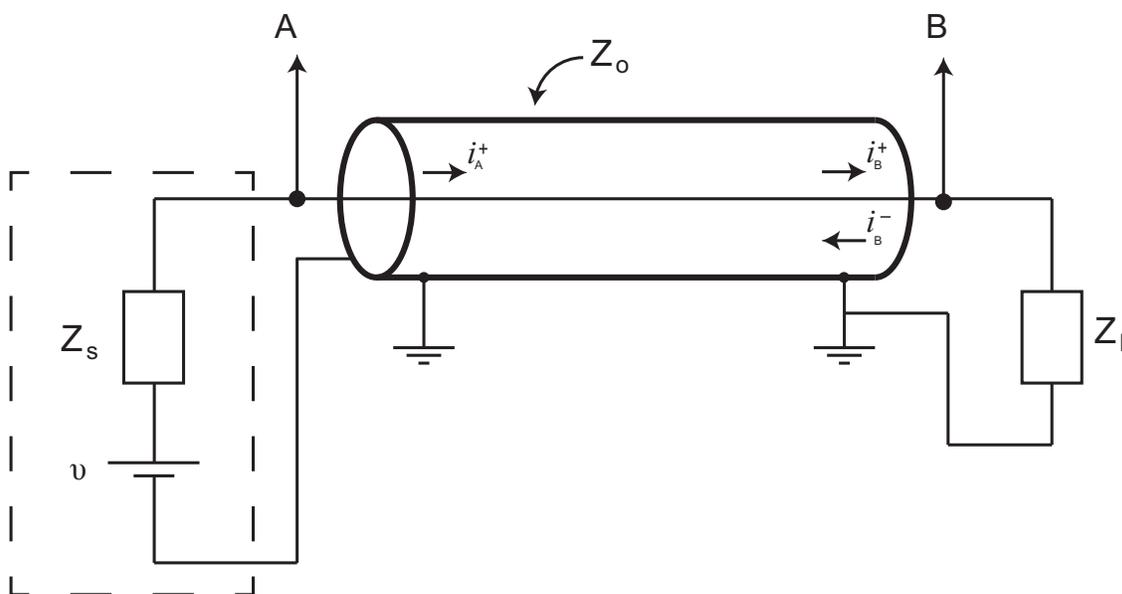
Figure 2: A diagrammatic overview of the experiment. The impedances  $Z_S$ ,  $Z_o$  and  $Z_L$  are associated with, respectively the source, cable and the load. The point **A** shows a test point where we could place an oscilloscope test probe and observe the resultant voltage stemming from the transmitted and reflected waves. The point **B** is the interface between the cable and the load. The dashed box indicates the source, in our experiment this is a pulse generator.
