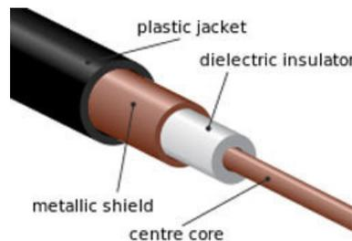
Figure 1: Cutaway of a general coaxial cable. The cable has two conductors separated by a dielectric. This construction imparts a characteristic impedance to the cable.
