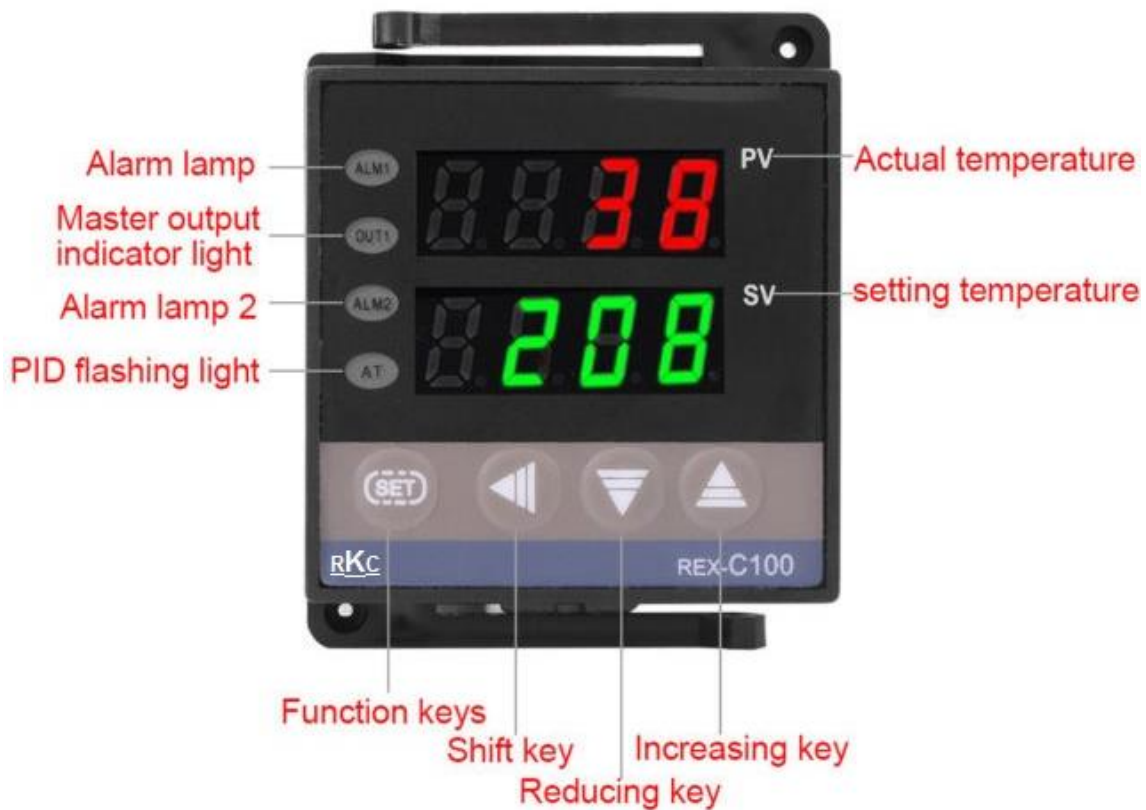
Figure 3: Front panel name and functions
