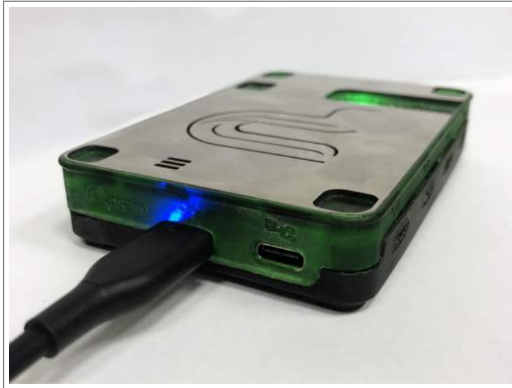
Figure 1.9: LED lights indicate that the PhysLogger device has been powered on and is ready to be used.
