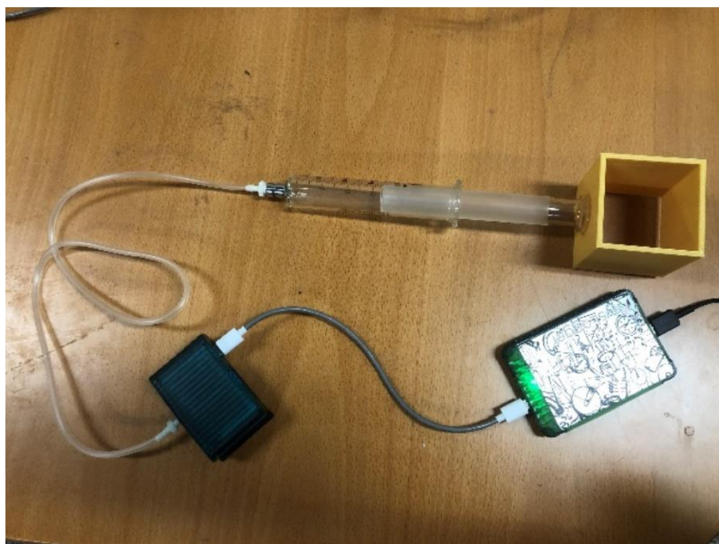
Figure 8: To investigate Boyle's law qualitatively, directly connect your syringe with PhysBar.
