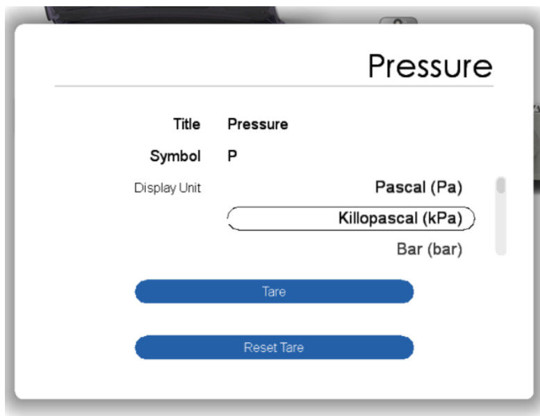
Figure 3: If PhysBar is configured with PhysLogger, you can find the Pressure quantity in Quantities Panel, clicking on that quantity opens this.
