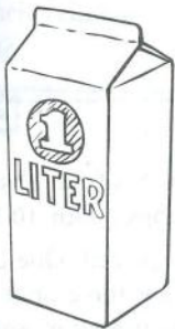
FIGURE 13.12 A liter of water occupies a volume of 1000\text{ cm}^3 , has a mass of 1 kg, and weighs 9.8 N. Its density may therefore be expressed as 1 kg/L and its weight density as 9.8 N/L. (Seawater is slightly denser, about 10.0 N/L).
