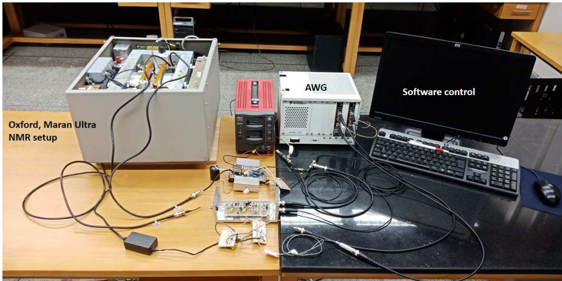
Figure 4.2: Complete NMR system with Maran setup. Controlled distribution of power through power supply runs the amplifier circuits.
