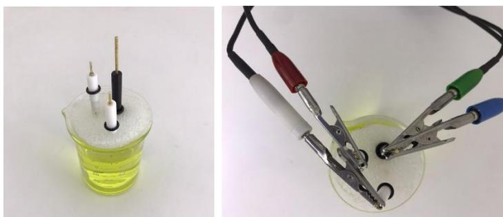
Figure 10: Experimental apparatus and electrode setup for CV measurement.
