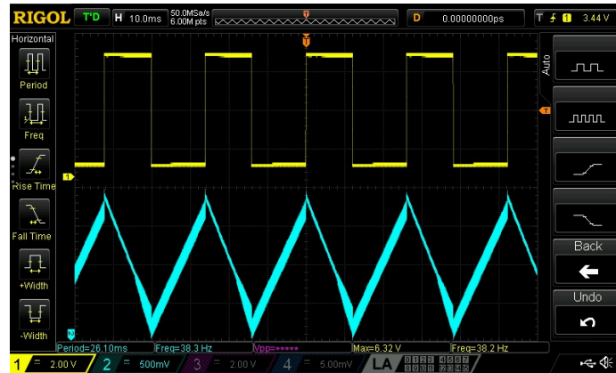
Figure 5: Output of the home-built function generator.
