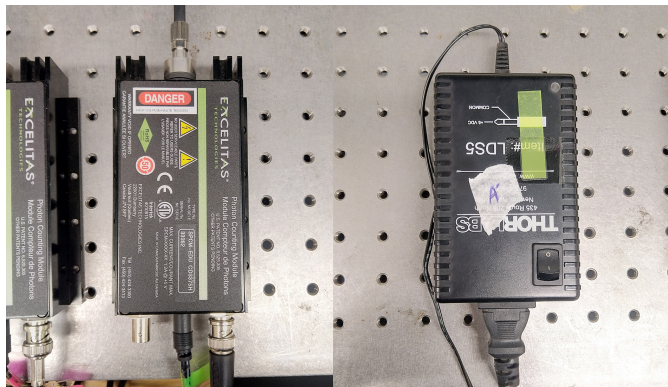
Figure 1.6: An SPCM on the left and its power supply on the right.
