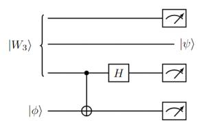
Figure 1: Quantum circuit for probabilistic teleportation.
