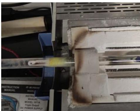
Figure 36: 1 inch tube fixed in the furnace, held in place using insulating material to counter heat loss around the ends and to fix the tube.
