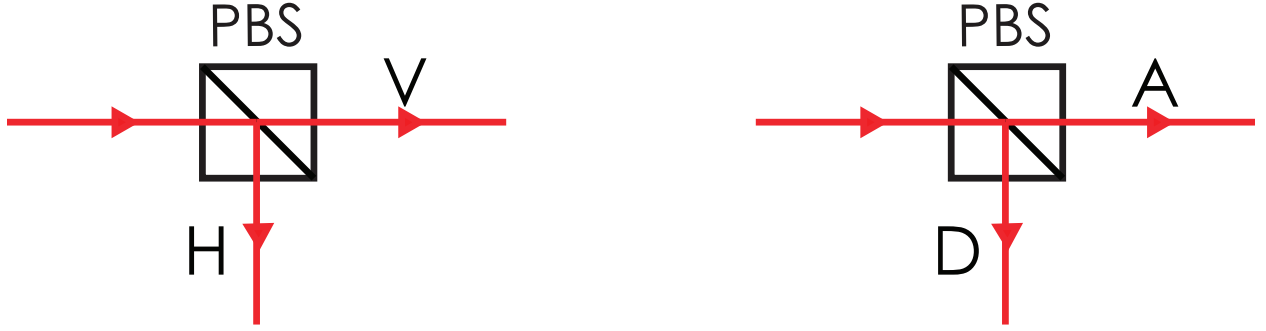
(a) A |H\rangle, |V\rangle PBS which transmits the vertically polarized photons |V\rangle and reflects the horizontally polarized photons |H\rangle .
