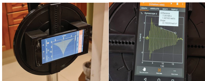
Fig. 4. Direct measurement of the moment of inertia; the period of oscillation was registered using the Phyphox app (left picture) and averaging over 10 oscillations (right picture).
