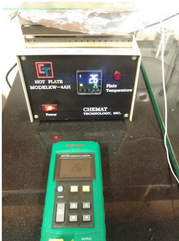
Calibration setup for a K-type thermocouple using thermocouple calibrator and a hot plate
