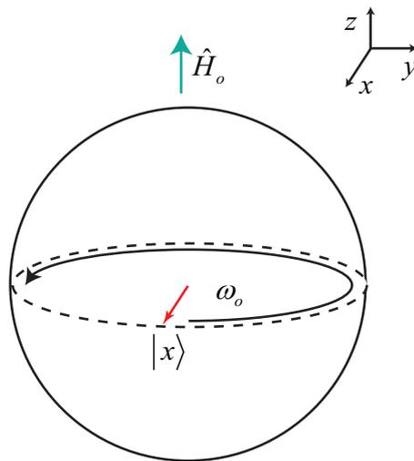
Figure 1.12: The spin angular momentum state vector precess with time
