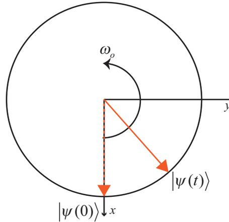
Figure 2.14: Top view showing the state precessing with frequency  $\omega_o$ .
