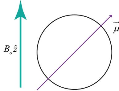
Figure 2.1: Magnetic moment of proton placed inside a uniform field
