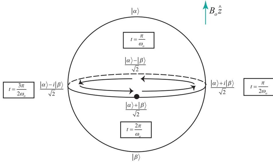
Figure 2.4: Representing precessional motion on the Bloch sphere.
