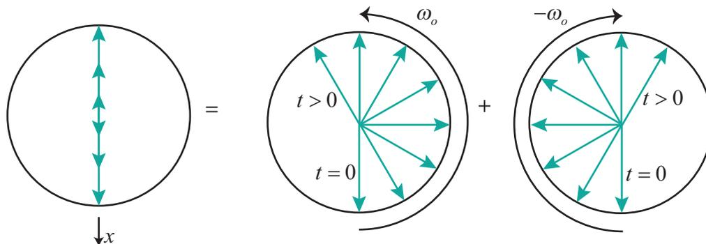
Figure 2.13: Top view of the rotating spin vector showing that reciprocating field along the  $x$ -axis is sum of two counter rotating fields.
