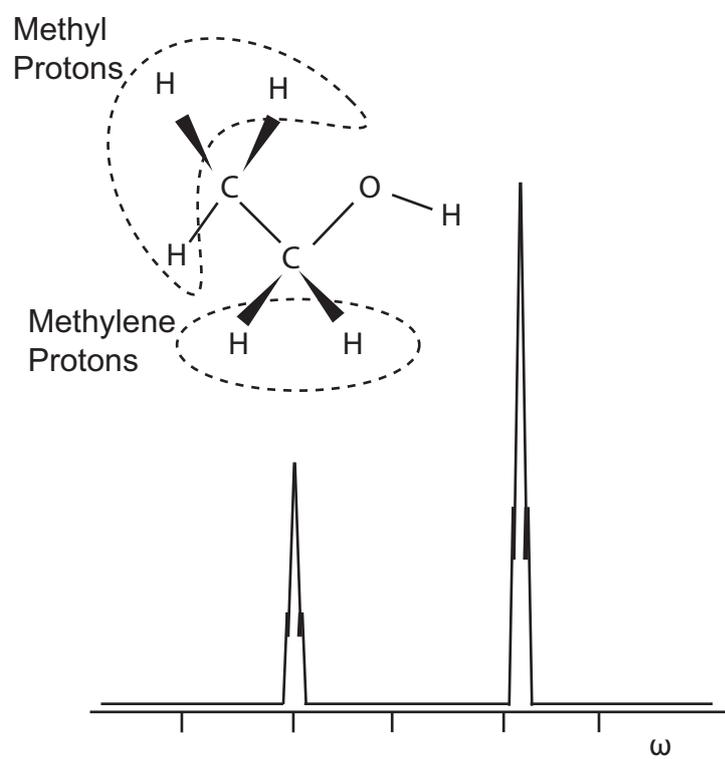
Figure 2.19: Proton spectrum of Ethanol
