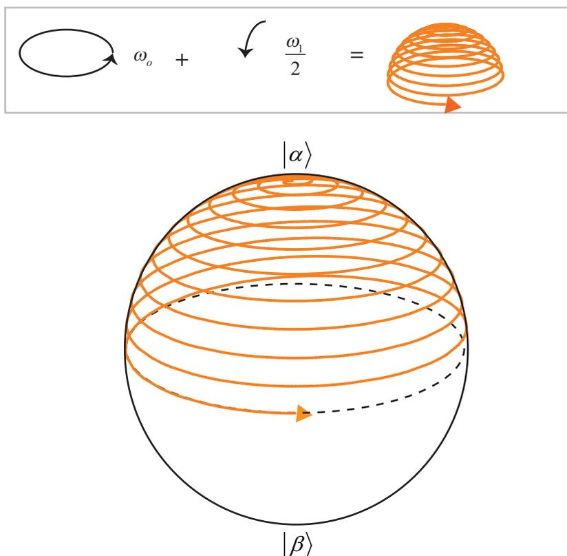
Figure 2.17: Precession with frequency  $\omega_o$  and nutation with frequency  $\omega_1$  in lab frame. The downward motion is still exaggerated. While we only have shown  $\approx 10$  azimuthal rotation inside a  $\pi/2$  rotation towards the equatorial plane, in real scenarios, the ratio of the number of azimuthal to polar rotation would be in the thousands.
