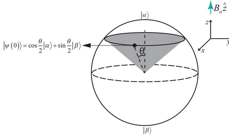
Figure 2.6: State in the  $x$ - $z$  plane is precessing with frequency  $\omega_o$  with a magnetic field applied in the  $z$  direction
