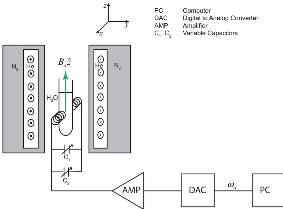
Figure 2.11: Oscillating magnetic field with Larmor frequency applied along the  $x$ -axis.
