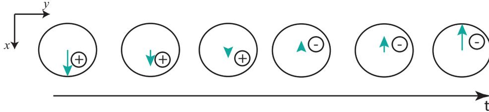
Figure 2.12: Top view of the vectorial field applied on the small coil. The field is sinusoidally reciprocating along the  $x$ -axis.
