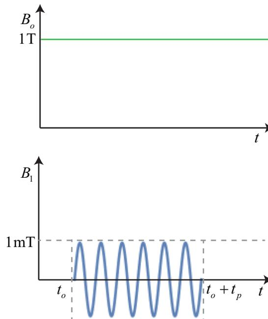
Figure 2.10: A timing diagram showing the fields  $B_o$  and  $B_1$ . The  $B_1$  field is oscillatory and turned on only for a finite duration  $t_p$ .
