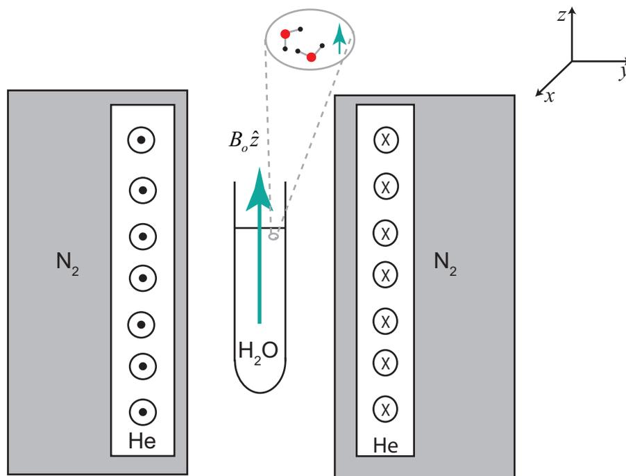
Figure 2.9: Magnetic field applied with the help of solenoid made of superconducting material. The superconducting coils are awash in liquid helium and surrounded by liquid nitrogen to soften the temperature gradient.
