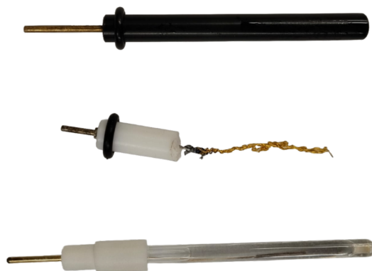
Figure 3.6: Experimental three-electrode used for electrochemical testing in our setup (top) Simple carbon working electrode used for testing, (centered) Gold wire used as counter soldered to a connector and (bottom) AgCl/Ag reference electrode used to maintain a constant reference potential.
