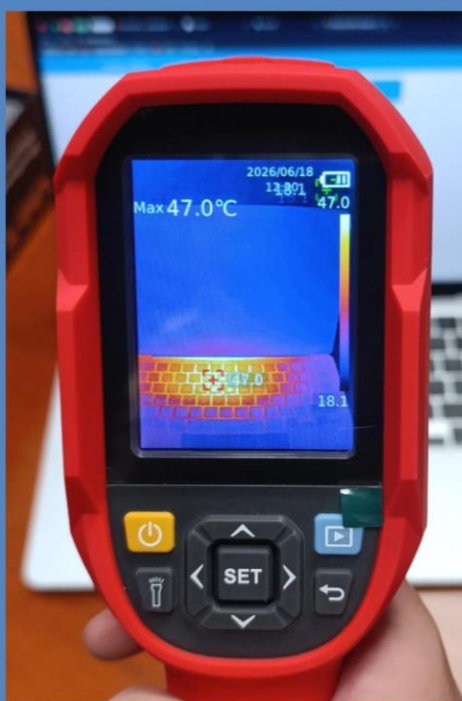
Figure 5. Thermal Inspection showing surface temperature of a laptop under maximum stress test inside an air conditioned room.
